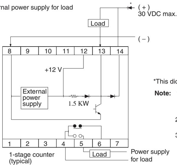
\*This diode is necessary if the supply voltage is below 12 V.
