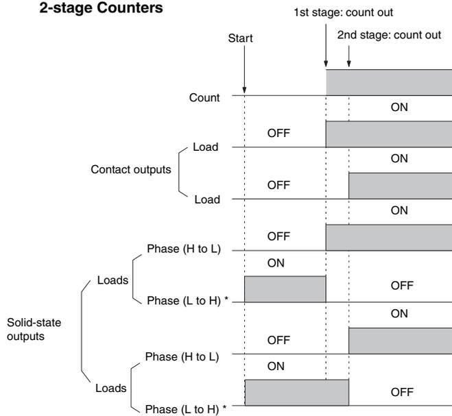
\* The operation of the load when the phase has been reversed.
