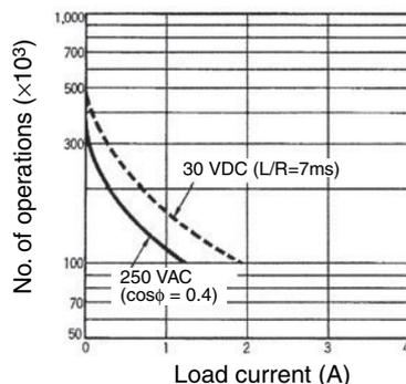
Reference: 0.15 A max. can be switched 100,000 times at 125 VDC ( $\cos\phi = 1$ ).
