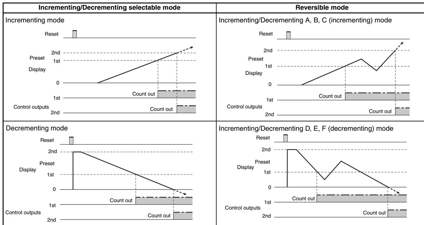
**Note:** Two-stage counters, set the counters so that the interval between 1st and 2nd count out will be more than 5 ms. For Incrementing/Decrementing switchable counters, only the 2nd value will be effective if the 1st value is larger than the 2nd value. The Incrementing/Decrementing Counters give outputs in the following order; 1st to 2nd to 1st to 2nd.
