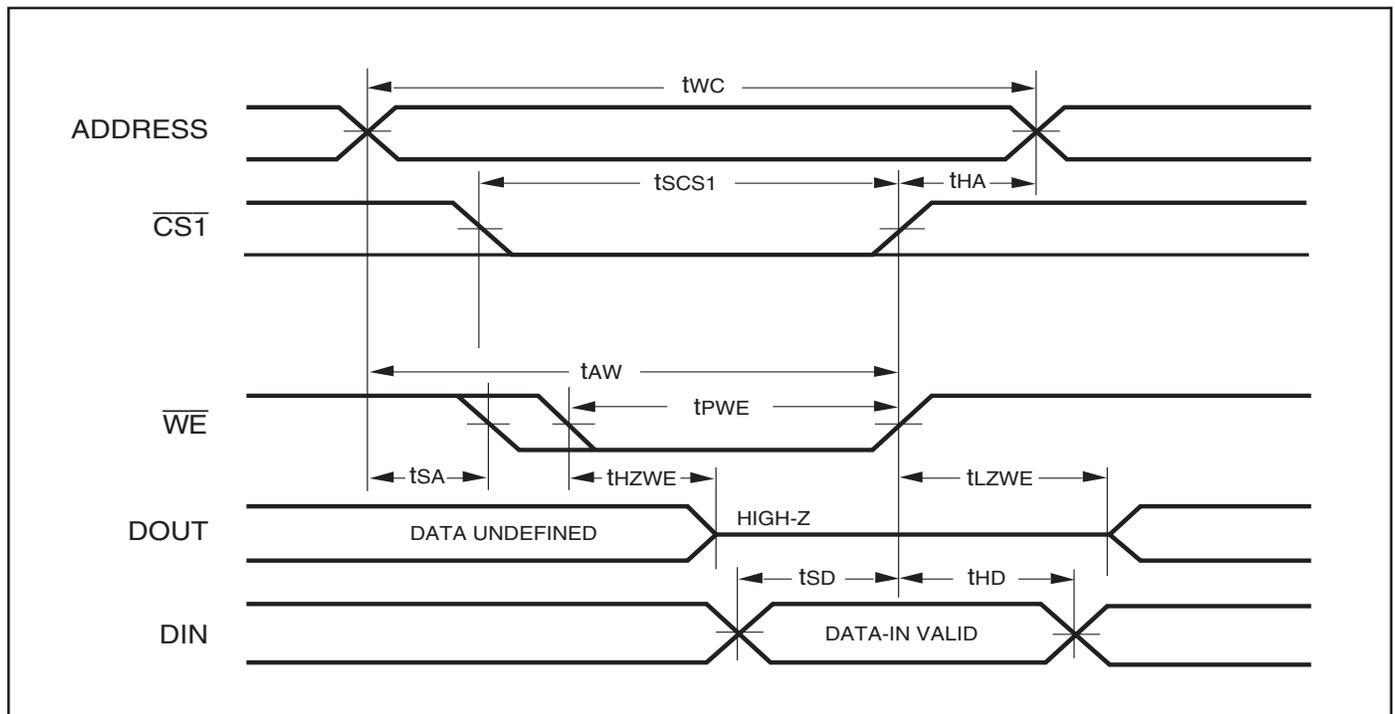
**WRITE CYCLE NO. 2** ( $\overline{WE}$  Controlled:  $\overline{OE}$  is HIGH During Write Cycle)
