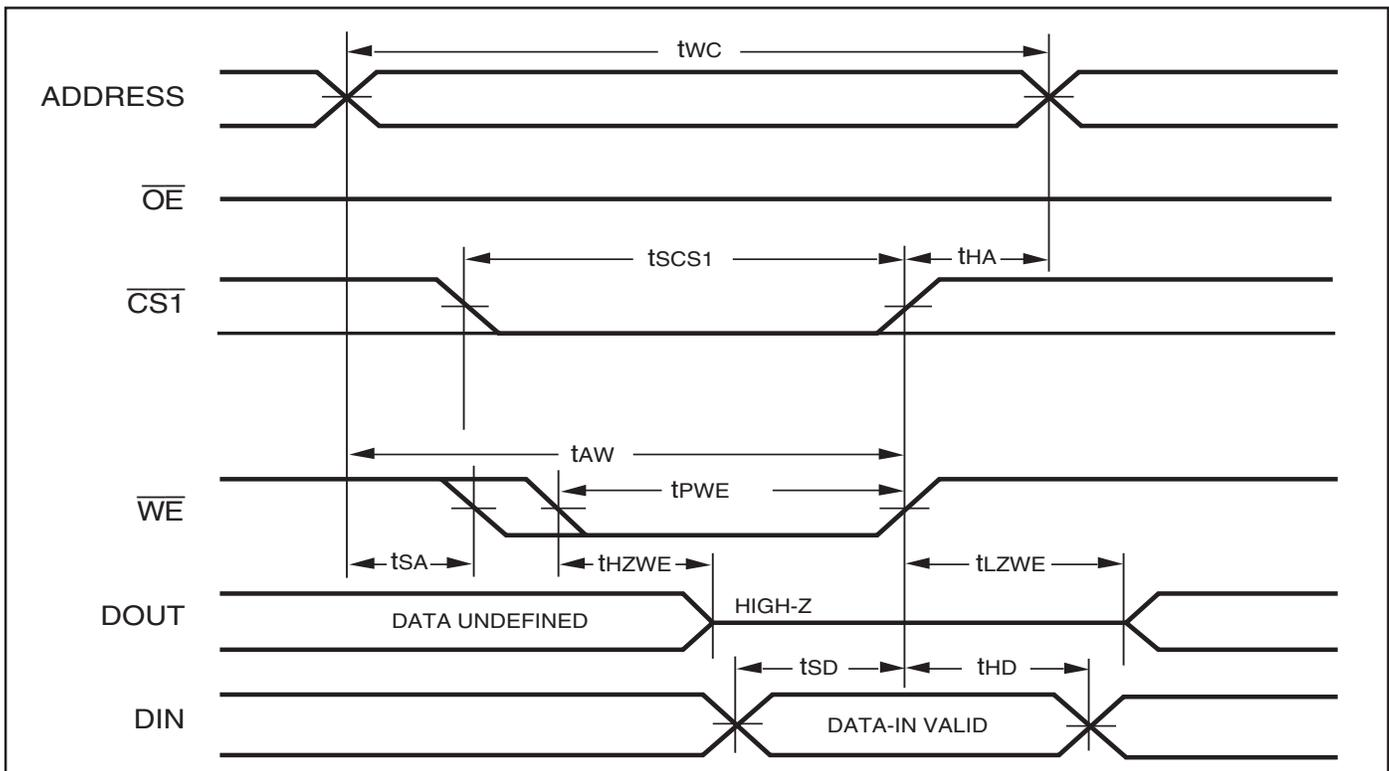
**DATA RETENTION SWITCHING CHARACTERISTICS**
