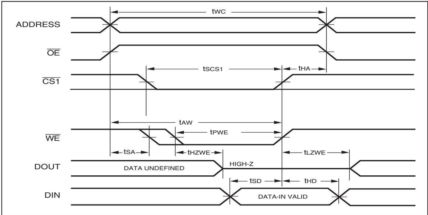
**WRITE CYCLE NO. 3** ( $\overline{WE}$  Controlled:  $\overline{OE}$  is LOW During Write Cycle)
