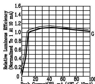
Fig2. RELATIVE LUMINOUS EFFICIENCY
