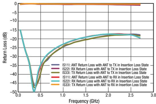
**Figure 13. Return Loss vs Frequency**
