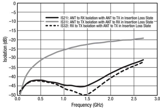
**Figure 11. Isolation vs Frequency**
