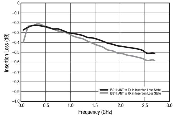
**Figure 10. Insertion Loss vs Frequency**
