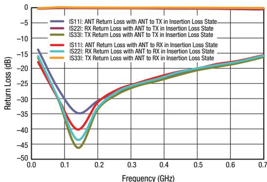
**Figure 7. Return Loss vs Frequency**
