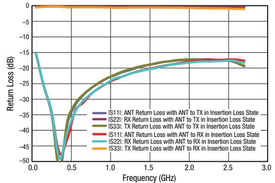
**Figure 14. Return Loss vs Frequency**
