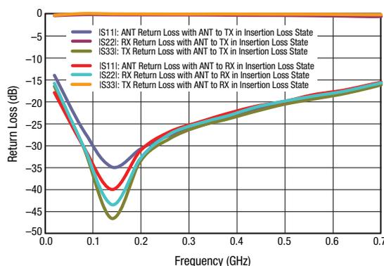
**Figure 8. Return Loss vs Frequency**
