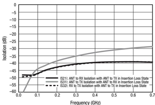
**Figure 5. Isolation vs Frequency**
