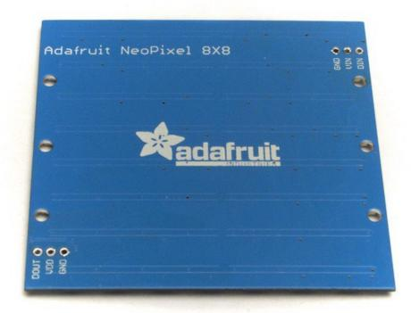
This is the NeoMatrix. It has two groups of three holes, labeled "DOUT / VDD / GND" on one side, and "GND / VIN / DIN" on the other side.
