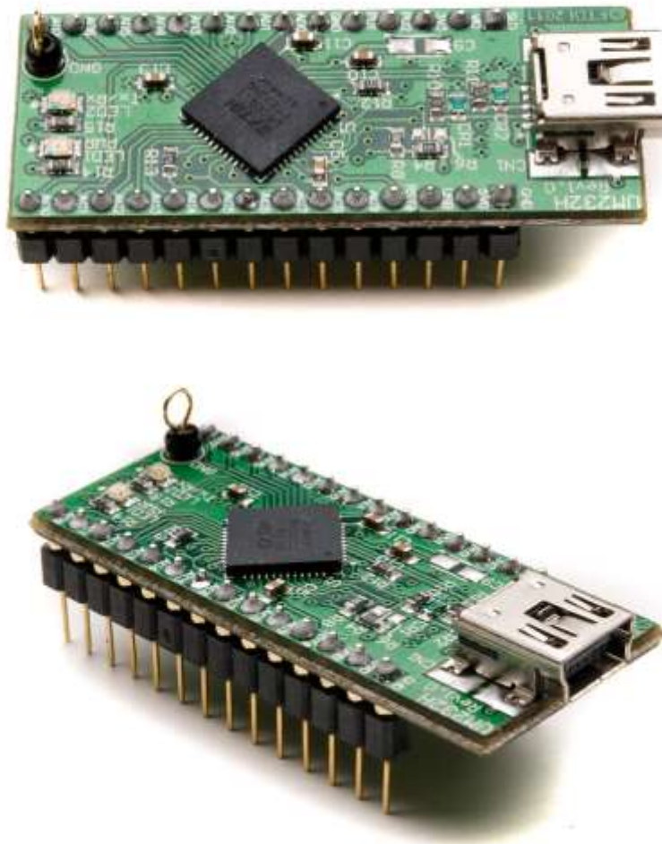
Figure 1 – UM232H USB to Serial/FIFO Development Module
