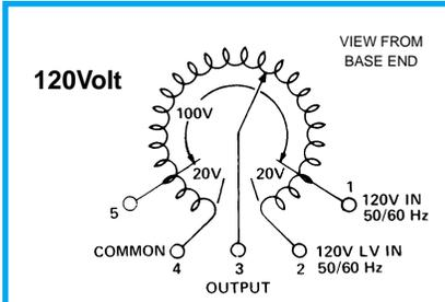
For opposite rotation interchange external connections from 1 to 5 and 4 to 2.
