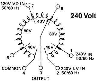
For opposite rotation interchange external connections from 1 to 5, 4 to 2 and 7 to 6.
