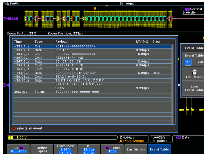
Event table for MIL-STD-1553 bus with all captured packets time stamped and in a tabular view.
