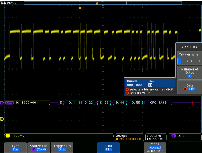
Triggering on a specific data value on the CAN bus.
