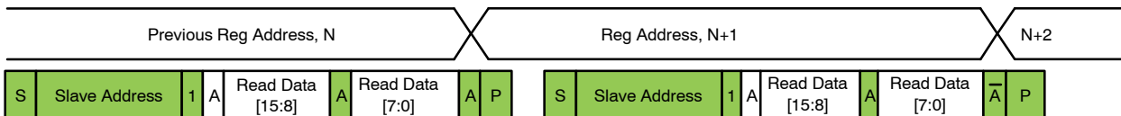
Figure 30. Single Read from Current Location
