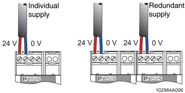
Figure 7 Individual/redundant supply
