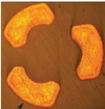
Au/Ni Barrier (Uniform plating thickness)
