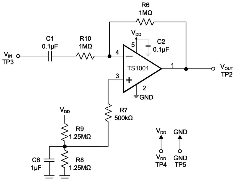
Figure 2. Inverting Configuration
