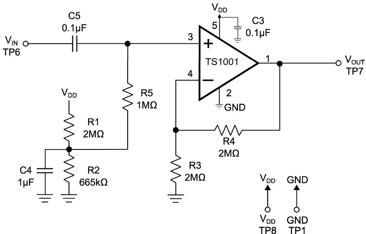
Figure 1. Non-Inverting Configuration
