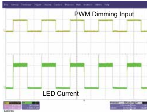
(a) PWM Dimming Performance Time Scale : 1ms/div
