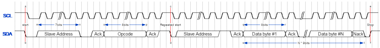
Figure 7: Read message transfer using a repeated start condition (I 2 C)
