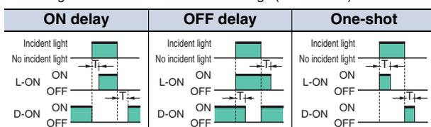
3. Control Output (AND, OR, Sync) and Timing Chart for Timer Settings (T: Set Time)
