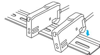
2. Slide the Amplifier Units together, line up the clips, and press the Amplifier Units together until they click into place.
