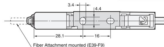
Note: When using E39-L143 Mounting Brackets, there will be small gaps between the Fiber Amplifier Units if they are mounted side by side.
