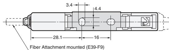
Note: When using E39-L143 Mounting Brackets, there will be small gaps between the Fiber Amplifier Units if they are mounted side by side.
