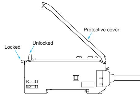
Note: 1. To maintain the fiber unit properties, confirm that the lock is released before removing the fiber units.
