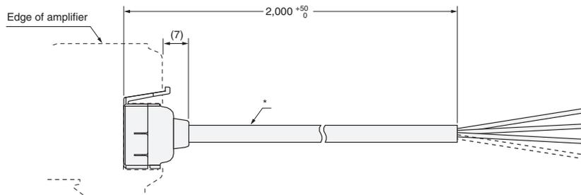
\* E3X-CN11: **4 dia.** cable / **3 conductors** / Standard length: 2 m (Conductor cross section: 0.2 mm<sup>2</sup> (AWG24), Insulator diameter: 1.1 mm)
