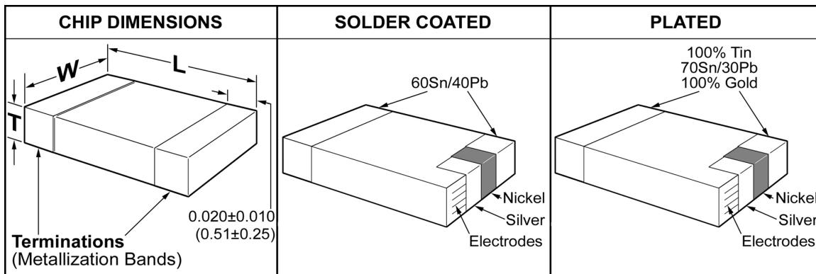
\*Add .38mm (.015") to the positive width and thickness tolerance dimensions and 0.64mm (.025") to the positive length tolerance dimension for solder coated(dipped) end metallization.
