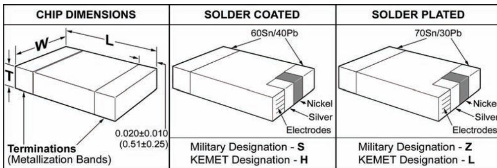
NOTE: For solder coated termination, add 0.015" (0.38mm) to the positive width and thickness tolerances. Add the following to the positive length tolerance: CKS51 - 0.020" (0.51mm); CKS52, CKS53 and CKS54 - 0.025 (0.64mm); add 0.012" (0.30mm) to the bandwidth tolerance.
