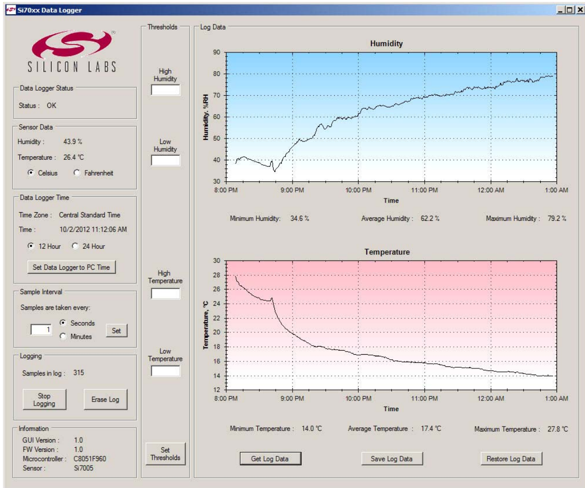
Figure 10. Data Logger Application
