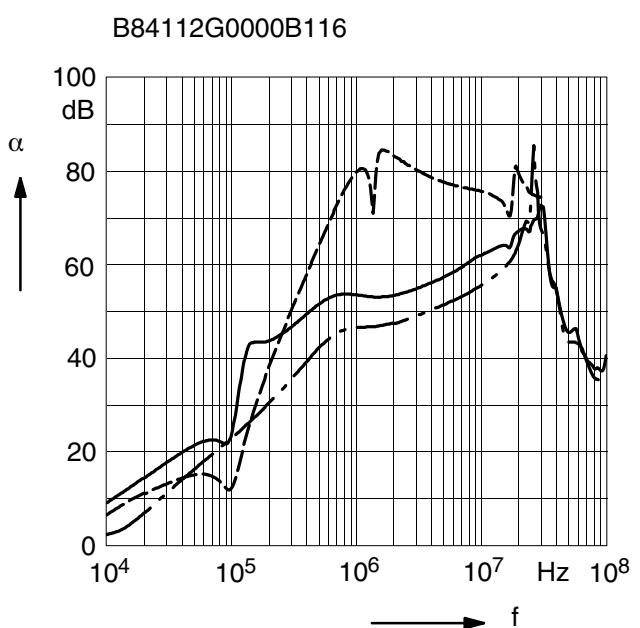
**Insertion loss (typical values at  $Z = 50 \Omega$ )**
