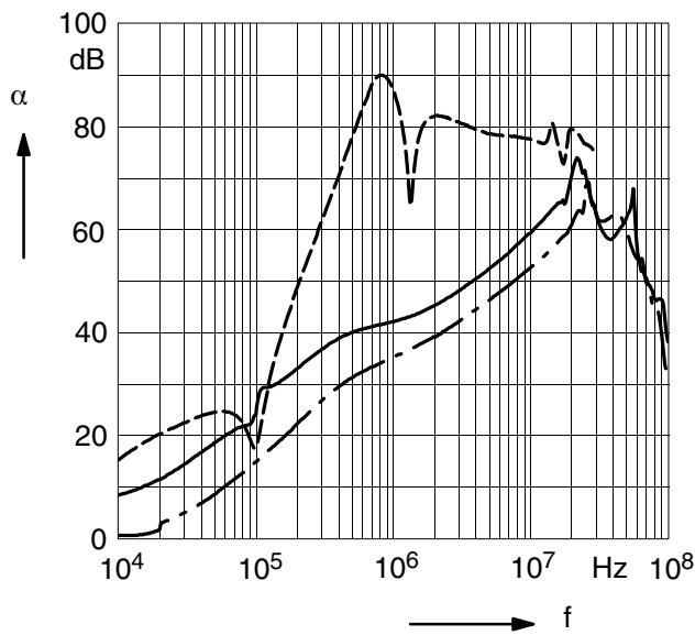
**Insertion loss (typical values at  $Z = 50 \Omega$ )**
