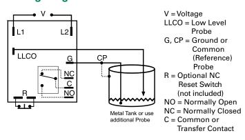
Relay contacts are isolated. Connect common to conductive tank. Additional probe is necessary for non-conductive or insulated tanks.
