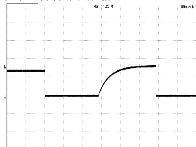
Figure 4: Vout start up with Vin on at 48Vin, 22A Iout, TOP:VIN, 20V/div, 200mS/div BOTTOM: VOUT, 5V/div, 200mS/div
