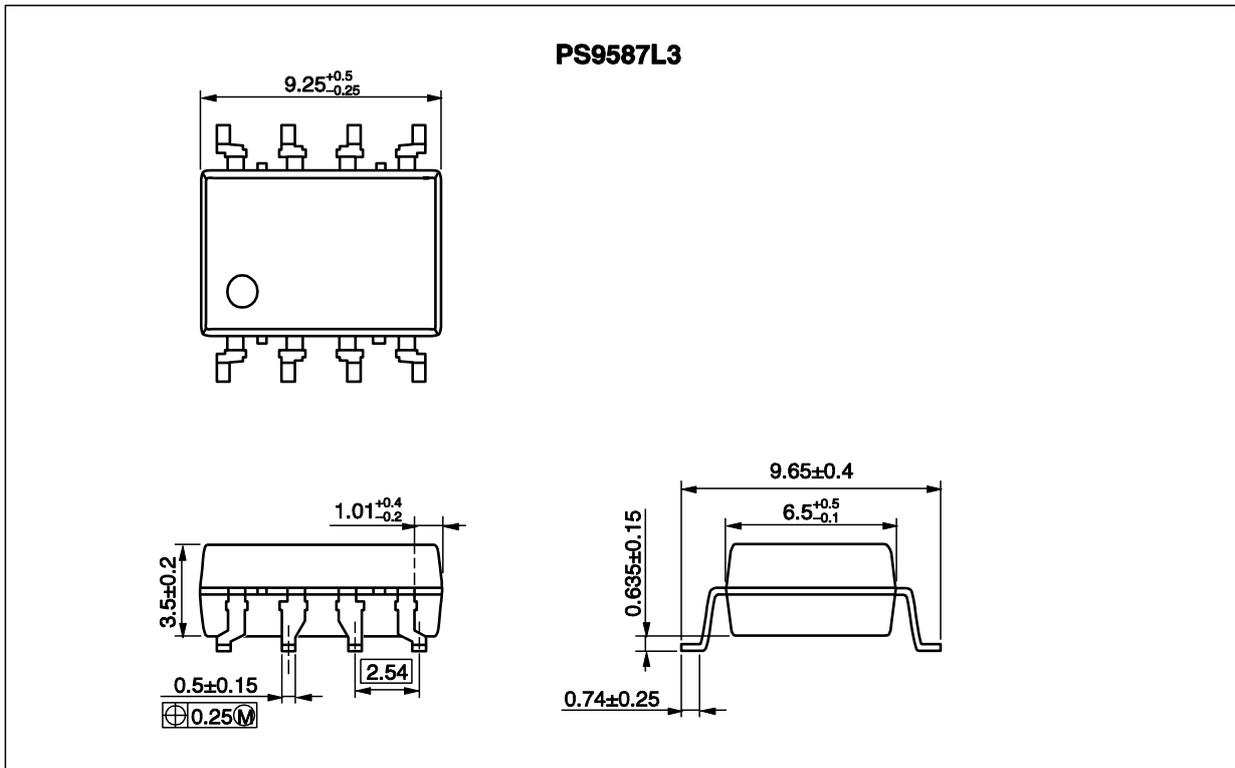
Lead Bending Type For Long Creepage Distance
