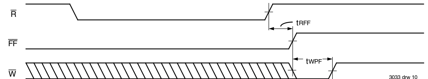
Figure 8. Minimum Timing for a Full Flag Coincident Write Pulse
