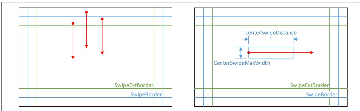
1. The user starts touching the surface with “n” fingers, where n is any number greater than zero. In the illustration above the user touches the surface with three fingers on the northern edge of the device.
