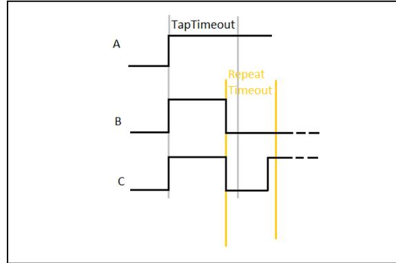
Once the user contacts the surface a timer starts running. If the user does not lift their finger(s) from the surface before TapTimeout has expired (as in part A of the drawing), the tap is considered aborted and the recognizer stops further processing. If the user lifts the finger without exceeding the timeout (as in part B and C), the recognizer considers it a tap.
