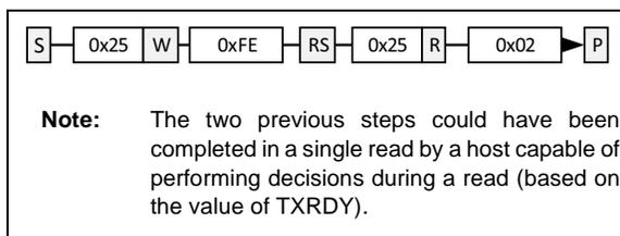
Reading address 0xFD auto-increments the address pointer to 0xFE, the stream buffer. Further bytes read will all be from within the stream buffer, maintaining the 0xFE address. The first byte read, 0x03, would indicate that three more bytes are within the stream buffer and may be read immediately.
