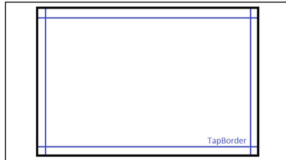
At least one finger has to be inside the area enclosed by TapBorder to start tap recognition, while the other fingers may be either outside or inside. So for a one finger tap the finger has to be inside, while for a two finger tap, one finger must be inside, while the second can be either inside or outside.
