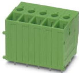
PCB terminal block, nominal current: 32 A, nom. voltage: 630 V, pitch: 7.62 mm, number of positions: 5, connection method: Front screw connection, mounting: Wave soldering, conductor/PCB connection direction: 90 °, color: green
