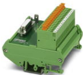
VARIOFACE module, with 15-pos. D-SUB socket strip and screw connection with knife disconnection, for mounting on NS 35/7,5 or NS 32
