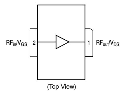
Figure 1. Pin Connections
