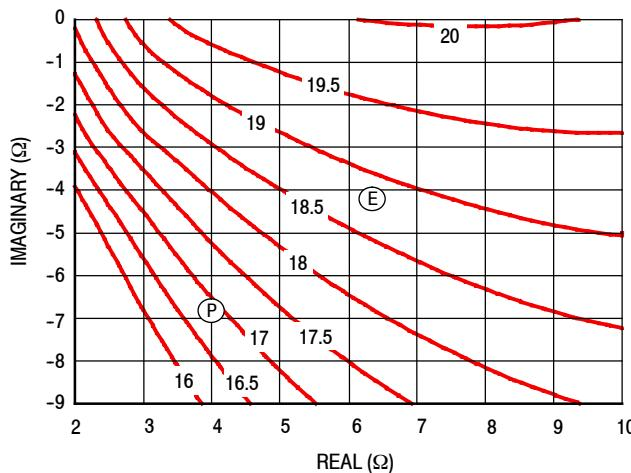
Figure 14. P3dB Load Pull Gain Contours (dB)
