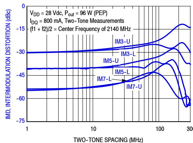
Figure 4. Intermodulation Distortion Products versus Two-Tone Spacing
