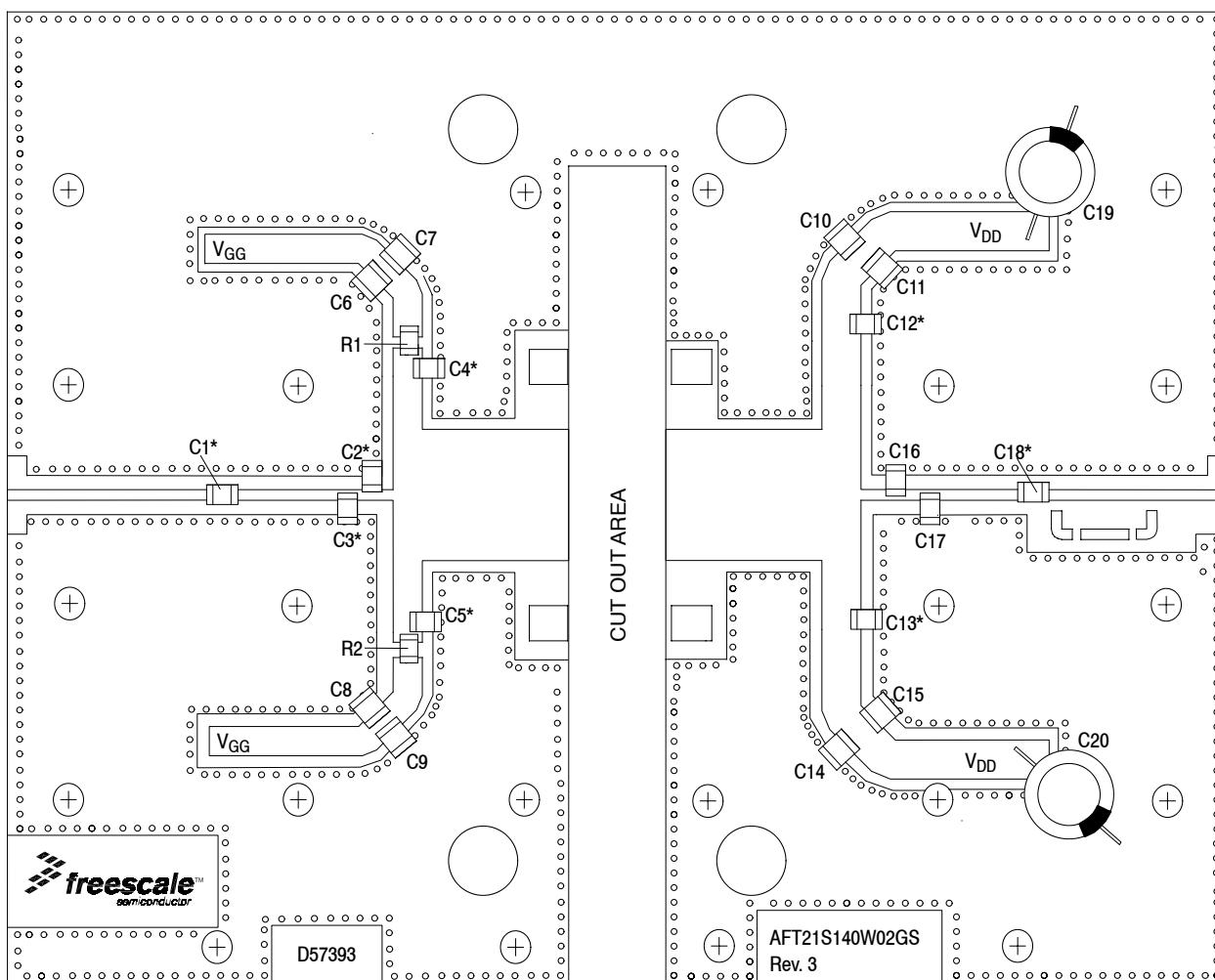
\*C1, C2, C3, C4, C5, C12, C13 and C18 are mounted vertically.
