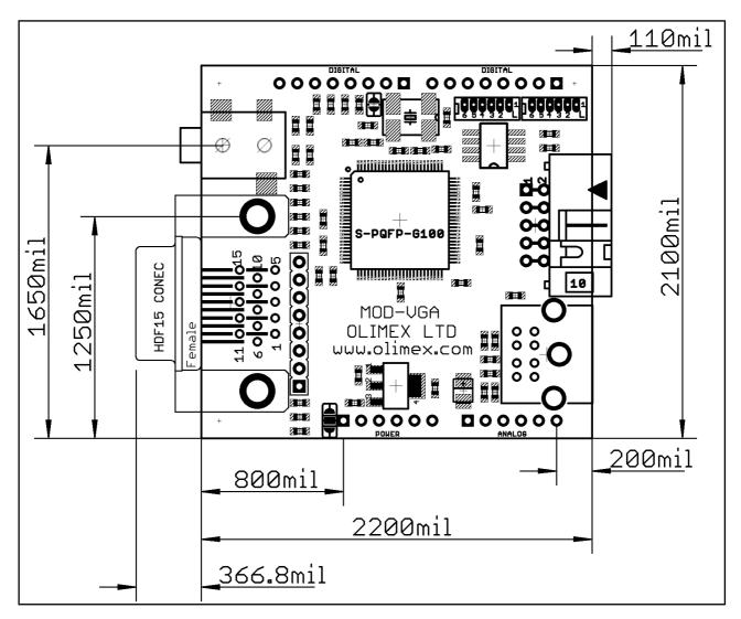
The two highest elements on the board are: VGA connector – 500mil; KEYBOARD connector – 500mil
