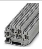
Component terminal block, Connection type: Spring-cage connection, Cross section: 0.08 mm² - 4 mm², AWG: 28 - 12, Nominal current: 22 A, Nominal voltage: 250 V, Length: 67.5 mm, Width: 5.2 mm, Color: gray, Assembly: NS 35/7,5, NS 35/15
