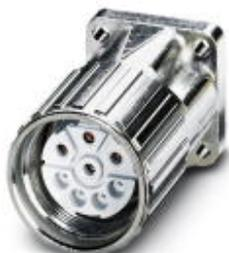
Device connector, front mounting with knurled nut, straight, Screw locking, M23, Number of positions: 5+PE, Type of contact: Socket, Crimp connection, Axial O-ring, 4xØ3,2, shielded: Yes, Flange dimensions: 26 mm x 26 mm, Cable diameter: 0 mm...0 mm
