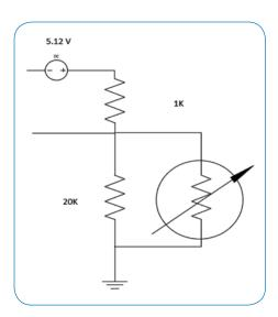
At this point, power across the NTC will be  $\sim$ 6.24 milliwatts. This will be the value needed for the power budget.
