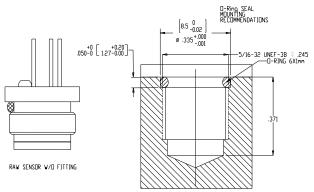
TYPICAL MOUNTING SOLUTION FOR RAW SENSOR
