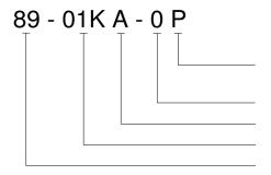
Electrical (P = Solder Pads, R = Ribbon Cable, C = Cable w/ Connector) Fitting Type Type (A = Absolute, S = Sealed Gage) Pressure Range Model
