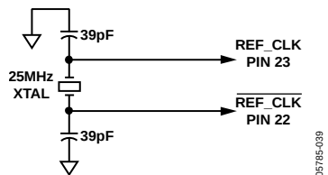
Figure 40. Crystal Configuration for Reference Clock Source
