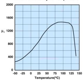
Measured on a 17/10/6mm toroid at 100kHz.
