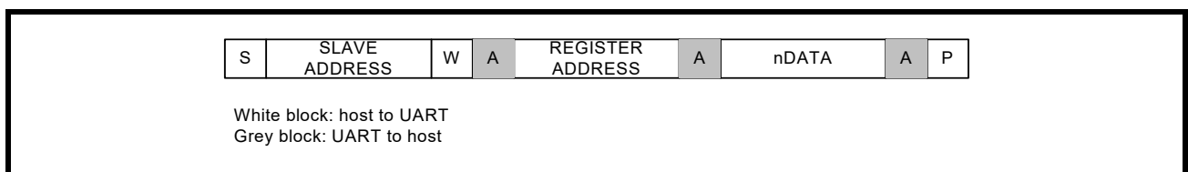
FIGURE 4. MASTER WRITES TO SLAVE (XR20M1170)
