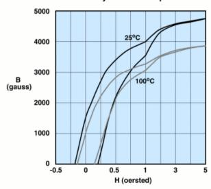
Measured on an 18/10/6mm toroid at 10kHz.
