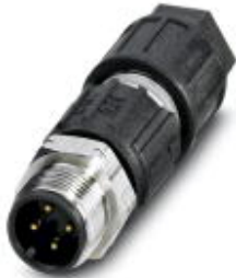
Sensor/actuator connector, male connector, straight, 4-pos., M12, A-encoded, QUICKON-ONE, high-grade steel knurl, maximum cable diameter of 6 mm
