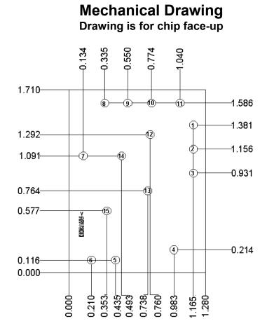
Units: millimeters Thickness: 0.38 Die x,y size tolerance: +/- 0.050 Chip edge to pillar dimensions are shown to center of pillar
