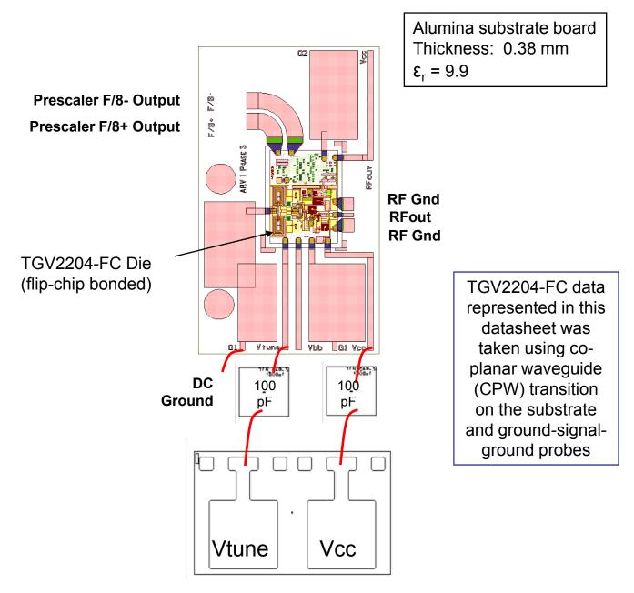
Die is flip-chip bonded / bumped to carrier
