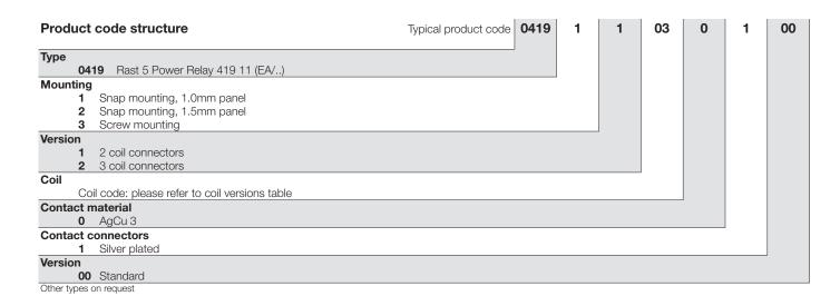
**Product code** Cont. material Version Cont.arrangement Coil Part number 0419 11 0301 00 Snap Mounting AgCu3 2 form A, 3-1415419-5 AC coil 2 NO 4-1415419-0 0419 11 1201 00 1.0mm plate DC coil 0419 11 1301 00 contacts 4-1415419-2 0419 31 0301 00 Screw Mounting AC coil 4-1415419-9
