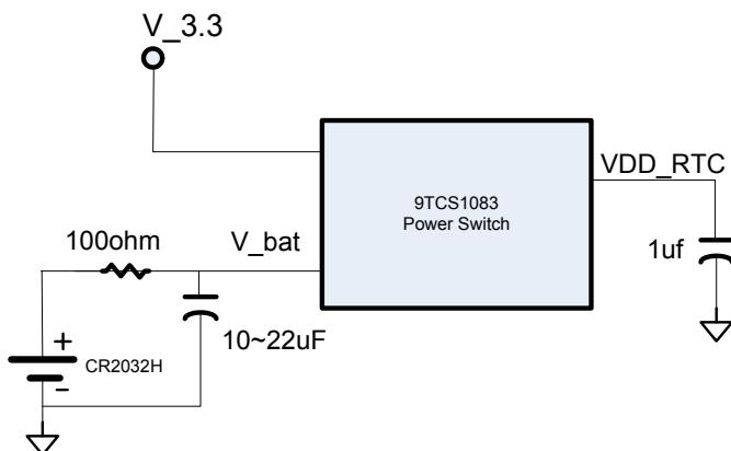
1. When the system is not power ON, V\_3.3 is not ready and IDT 9TCS1083 is powered with the coin cell battery. The 32kHz comes from the DCO with the digital calibration to keep the accuracy.
