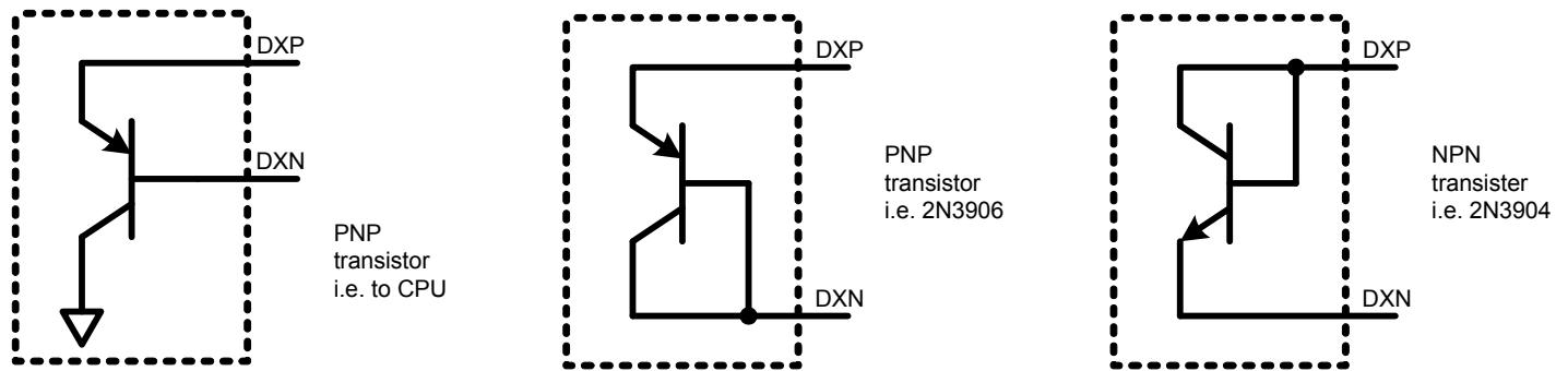
When the thermal sensor is used in a noisy environment, a capacitor can be connected across DXP and DXN to provide some noise filtering capabilities. However, large capacitances affect the accuracy of the temperature measurement. A maximum capacitance of 300pF can be used to help mitigate the noise.
