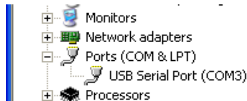
Figure 3-8 COM Port Assignment
