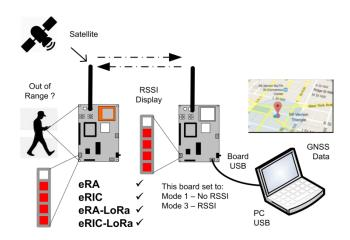
In this mode, the GNSS module, the PIC microcontroller and the eRIC/eRA modules are interconnected by software. Software in the PIC microcontroller discovers the Baud rate of the chosen eRIC/eRA modules and sets the microcontroller UART to match that of the modules.
