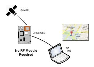
This mode allows the GNSS module serial data to be directly accessed by connecting a cable between the board GNSS micro USB connector (note position) and a PC USB port.
