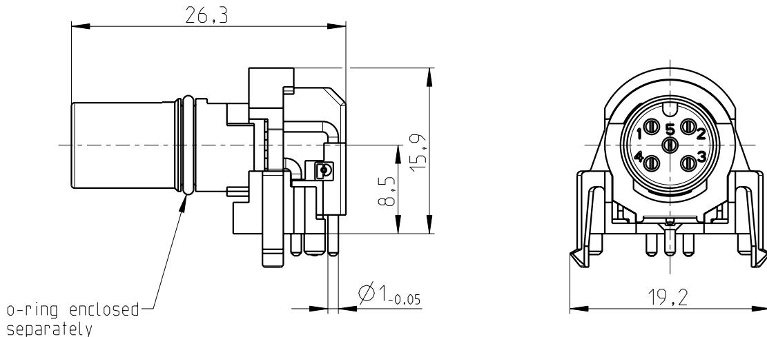
All specified data refers to the mounted M12 installation plugs >IP54 and requires that the connector pair be correctly plugged and locked. Influences from wires, cables or PCB mounting are also to be taken into consideration.
