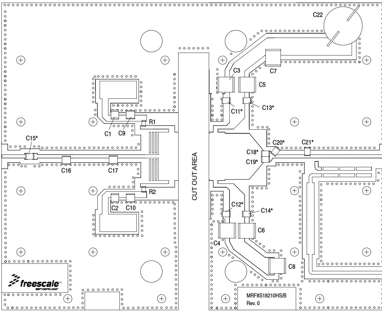
\*C11, C12, C13, C14, C15, C18, C19, C20, and C21 are mounted vertically.
