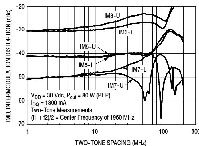
Figure 4. Intermodulation Distortion Products
