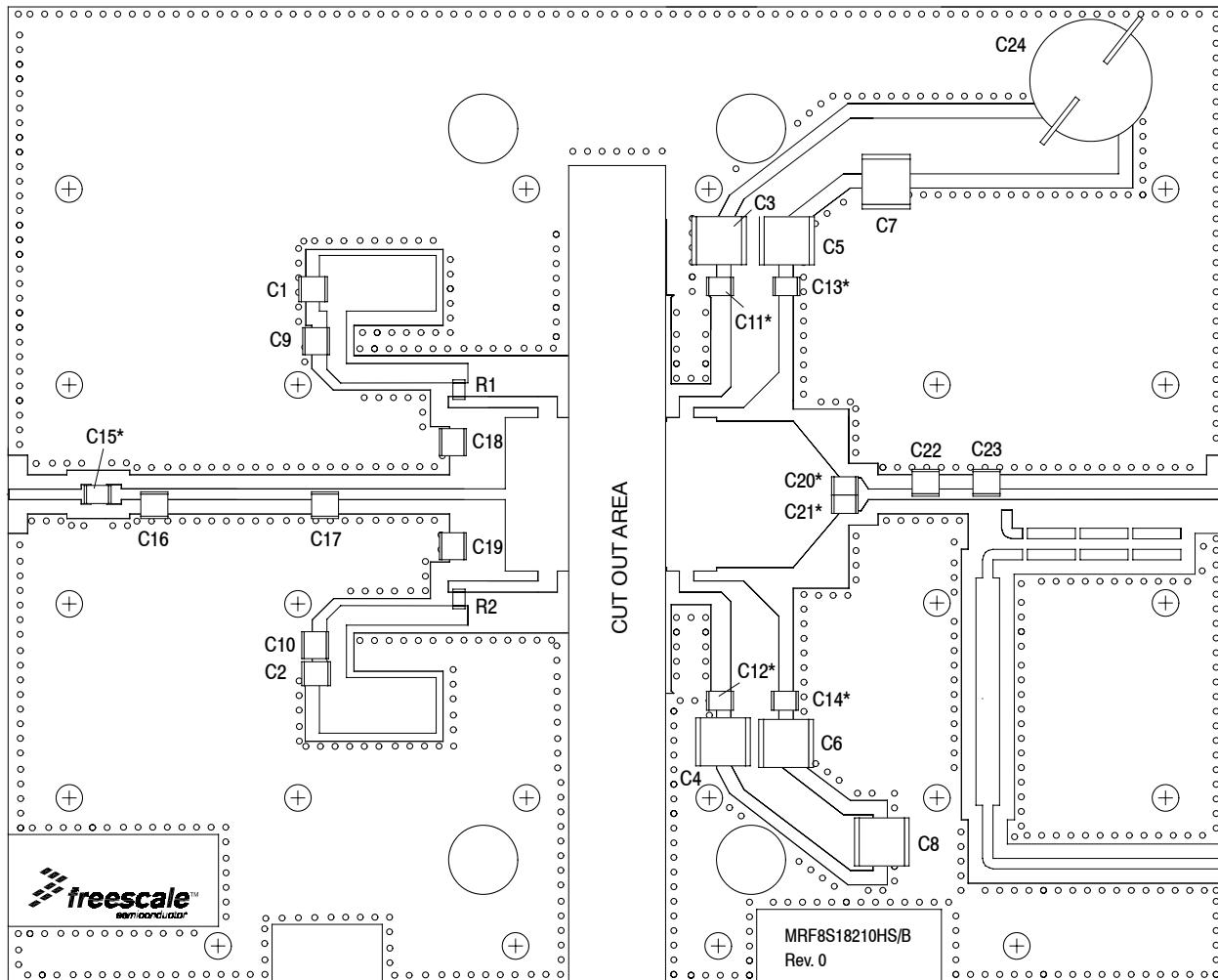
\*C11, C12, C13, C14, C15, C20, and C21 are mounted vertically.
