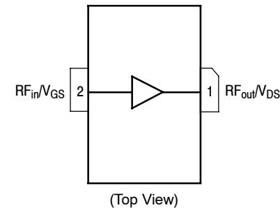
**Figure 1. Pin Connections**
