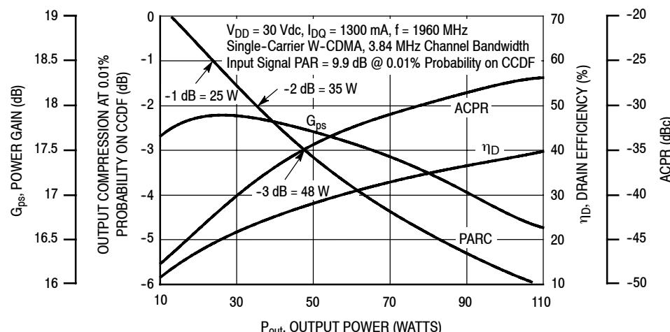
Figure 5. Output Peak-to-Average Ratio
