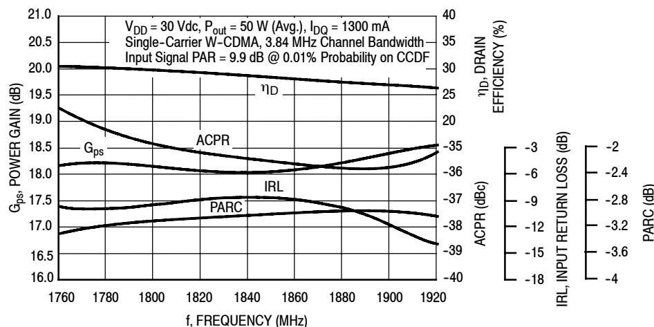
**Figure 14. Output Peak-to-Average Ratio Compression (PARC)**
