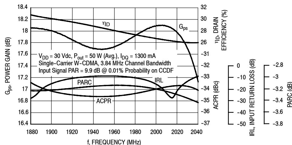
Figure 3. Output Peak-to-Average Ratio Compression (PARC)
