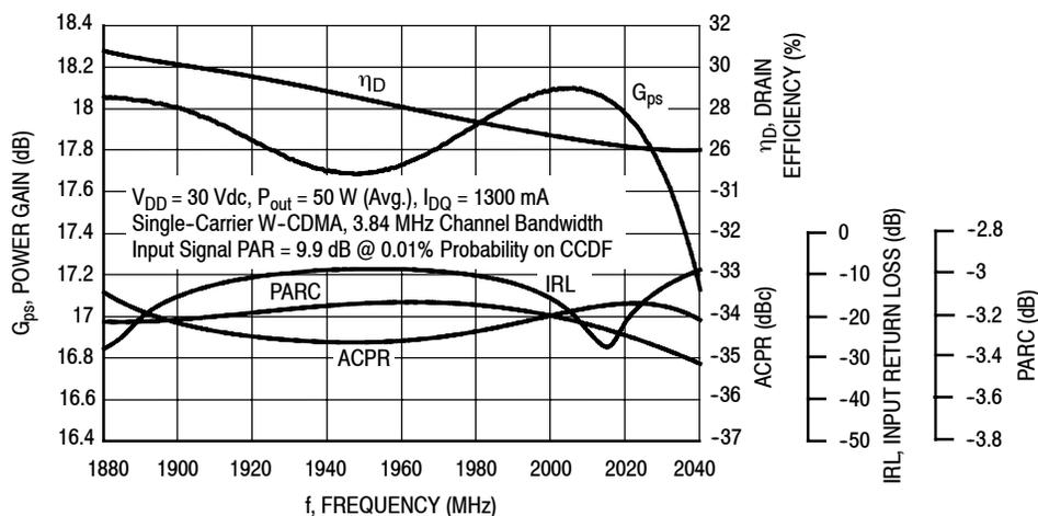
**Figure 3. Output Peak-to-Average Ratio Compression (PARC) Broadband Performance @ P<sub>out</sub> = 50 Watts Avg.**
