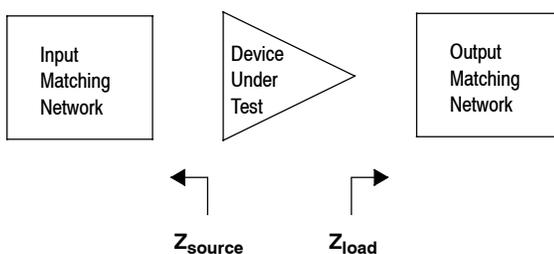
**Figure 10. Series Equivalent Source and Load Impedance**
