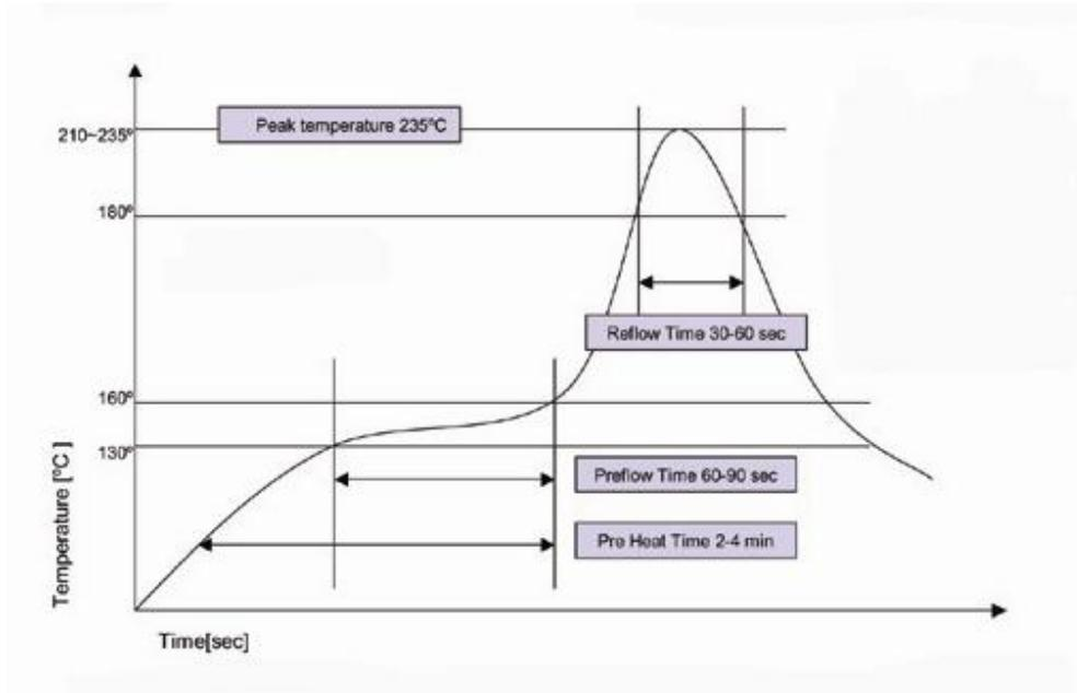
Figure 5 – Low Temperature Solder Reflow Thermal Profile
