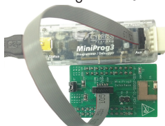
Fig 3: Programming/Debugging with MiniProg3
