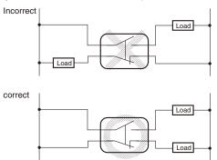
Connect the load to the same polarity.
