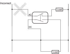
Do not design a circuit where voltage is imposed between contacts, otherwise contact weld may result.
