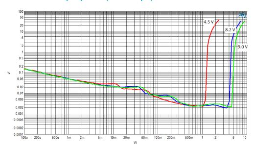
Figure 3: THD versus output power (8  $\Omega$  + 33  $\mu$ H)
