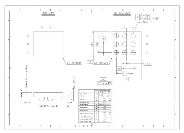
Figure 22: DA7202 package outline drawing (9-bump WL-CSP 0.5 mm pitch)
