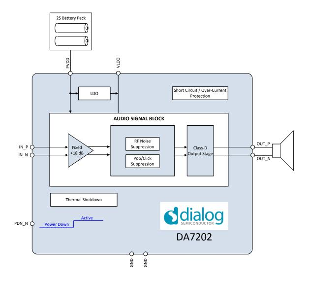
Figure 1: DA7202 block diagram
