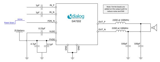
Figure 20: Layout of recommended external components and their values
