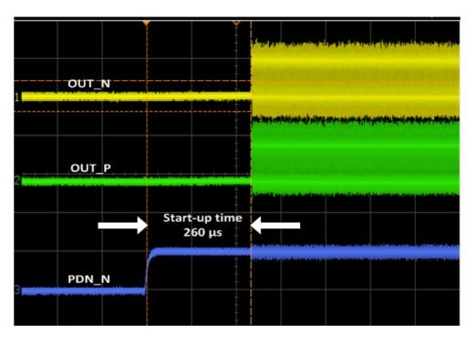
Figure 15: Start-up timing (260 µs from asserting PDN\_N to valid output)
