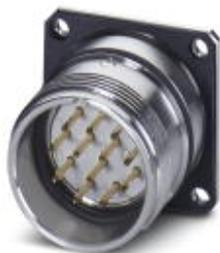
Device connector for rear wall, straight, Screw locking, M23, No. of pos.: 8+1, type of contact: Pin, Solder-in connection, Flat gasket, 4xM3, Panel thickness min.: 2.7 mm, Panel thickness max.: 3.5 mm
