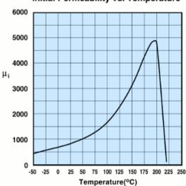
Measured on a 13/8/6mm toroid at 100kHz using the HP 4275.
